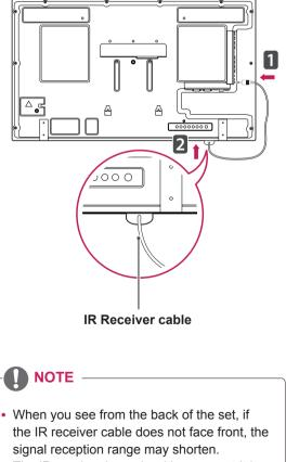
• The IR receiver is made with a magnet. It is detachable at the bottom (typical installation) or back (wall installation) of the set.
